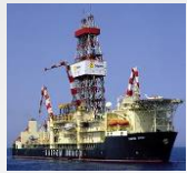
Saipem 10000 Ultra-deepwater Drillship WD 3,000 m
